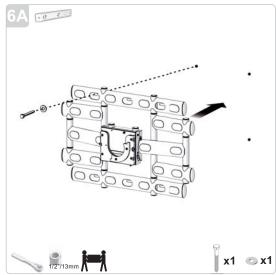
With minimum two people place the PFW6857 wall plate assembly and secure to the wall using the top center hole of the wall plate.
