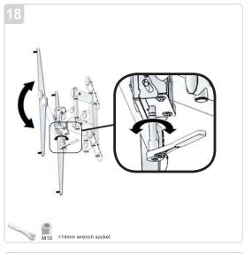
The PFW6857 has a unique "load offset adjustment" feature that allow for the heavier weight displays to be tilt corrected past base center back to level from top to bottom. With personal lifting gently "out " on the bottom of the display a 9/16" (14mm) socket may be used to increase or decrease the tilt feature of the mount.
