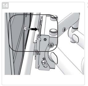
With the cross bar fully seating into the receiver reinstall the 6mm safety knurl knob.
