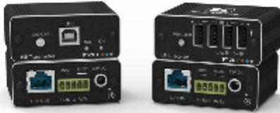
**PT-2UT/R** is a comprehensive, extended-reach HDBaseT extender kit for USB 2.0, RS-232 and audio signals and 2-way powering over twisted pair. The PT-2UT transmitter converts the USB input signal into an HDBaseT signal. The PT-2UR receiver converts the transmitted HDBaseT signal into a USB signal.
