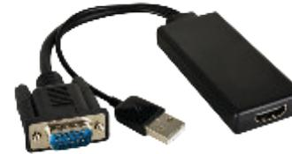
**ADC-GM/HF** is a VGA to HDMI™ adapter cable. This active cable converts an analog VGA signal to a digital HDMI signal. A USB-A connector enables inputting audio to the HDMI output and powering the cable.
