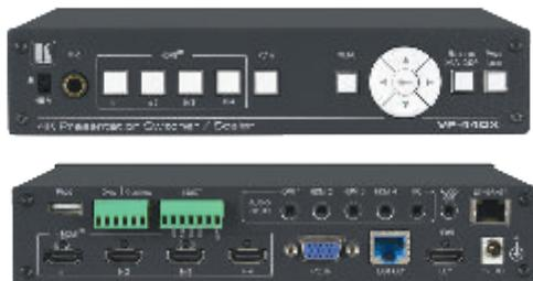
VP-440X is a high-performance 18G 4K HDR presentation switcher/scaler with four HDMI inputs and one computer graphics (VGA) input. It scales the video, embeds the audio, and outputs the signal to two identical outputs - one HDMI and one HDBaseT - together with an analog stereo audio output.
