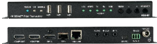
**KDS-8F** is a high-performance, zero latency, 4K@60Hz (4:4:4) video streaming transceiver for streaming via Ethernet over single-mode and multi-mode optical fiber. **KDS-8F** can be set as either an encoder or decoder. As an encoder, it encodes and streams the HDMI or DisplayPort input along with IR, RS-232, analog audio and USB, over an IP network. As a decoder, it receives the encoded signal and decodes it for output.
