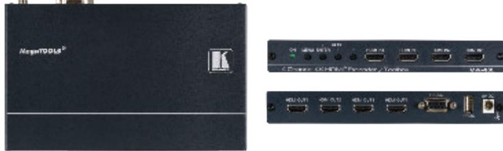
VA-4X is a versatile 4K@60Hz (4:4:4) HDMI multi-channel extender that equalizes and reclocks TMDs data before re-transmitting the signal, thus increasing the HDMI cable range for all 4 outputs. It is a true 4-channel HDMI "Toolbox", with functionality including 4 independent test-pattern generators, chroma sub-sampling down-conversion and EDID management options.
