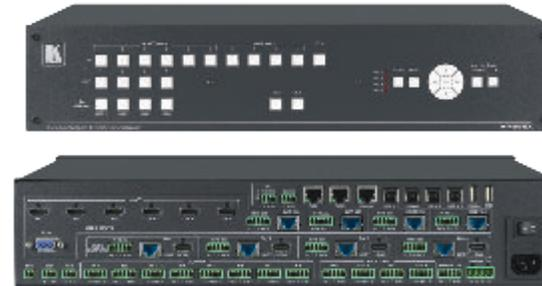
**VP-558X** is a high-performance 11x4 ProScale presentation scaler/matrix switcher outputs four independent scaled images to both HDMI and HDBaseT outputs. **VP-558X** supports digital and embedded audio and features six HDMI inputs, four HDBaseT inputs, an analog VGA input, and a 4x1 USB switcher. **VP-558X** also includes a microphone input, independent stereo audio outputs, a monitor output, an amplified speaker output, and audio DSP features.
