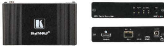
**675T** is a high-performance HDMI fiber transmitter for ultra-reach extension of 4K60Hz (4:4:4) HDMI signals over multi-mode or single-mode fiber optic. **675T** converts the HDMI input signal to an optical signal that is transmitted over a fiber optic cable to a compatible receiver that converts it back to an HDMI signal.
