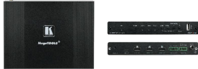
**VP-451** is a high-performance 18G 4K digital scaler for HDMI and USB-C signals. The unit up-scales, down-scales, and cross-scales to resolutions up to 4K@60 (4:4:4). The output resolution can be set to automatically follow the native resolution of the sink or set manually to a custom resolution.
