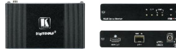
**675R** is a high-performance HDMI fiber receiver for ultra-reach extension of 4K60Hz (4:4:4) HDMI signals over multi-mode or single-mode fiber optic. **675R** receives the transmitted optical signal from a compatible transmitter and converts it to an HDMI signal.
