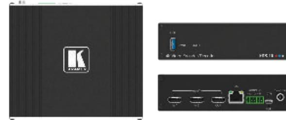
**KDS-10** is a high-performance, multi-standard streaming transceiver for streaming 4K@60Hz (4:4:4), HDR, HDCP 2.2 video signals via Ethernet over copper cable. **KDS-10** can be set as either an encoder or decoder. As an encoder, it encodes and streams one or two HDMI inputs over an IP network. As a decoder, it receives the encoded signal, decodes it and outputs it to an HDMI output.
