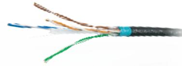
**BCP-HDKat6** is a high-performance unified CAT6 Plenum rated cable that handles all Pro AV and IT signals over four overall screened twisted pairs. This F/UTP CAT6 cable uses HDBaseT and Kramer's DGKat™ technology to pass video signals of up to 4K@60 (4:4:4) resolution. **BCP-HDKat6** is also ideal for LAN applications.
