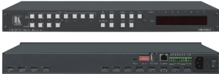
**VS-48H2** is a high-performance 4x8 matrix switcher for 4K@60Hz (4:4:4) HDR signals and digital audio routing. It reclocks and equalizes the signals and can route any one of 4 HDMI, HDCP-compliant sources (selectable) to any or all outputs simultaneously. **VS-48H2** offers unmatched audio flexibility where any embedded digital audio input can be routed to any digital output in addition to eight ARC sources to produce an equivalent 12x10 audio matrix.
