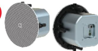
Tavor 6-CNet is a high-performance, in-ceiling, PoE powered speaker with 2 channels of Dante input. This active speaker receives audio and powering via an Ethernet cable.
